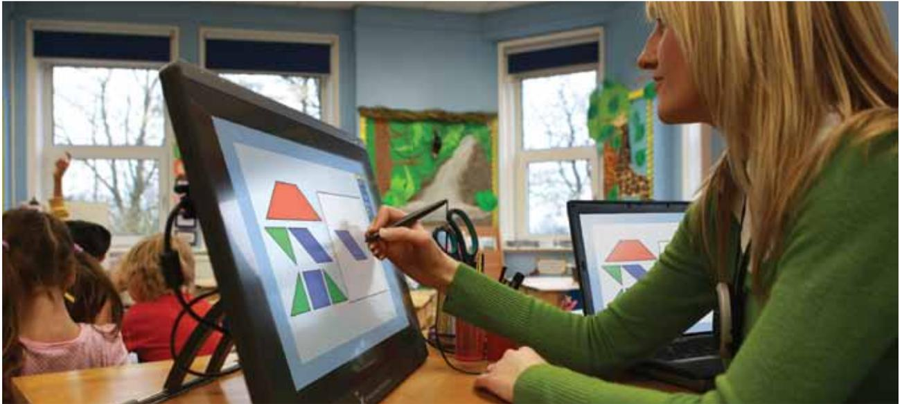
The **ActivPanel** is an **interactive display monitor** that connects to a computer and a projector and performs all mouse and display functions. Using the ActivPanel, a presenter can open, view and control any software application using a pen-like stylus.
